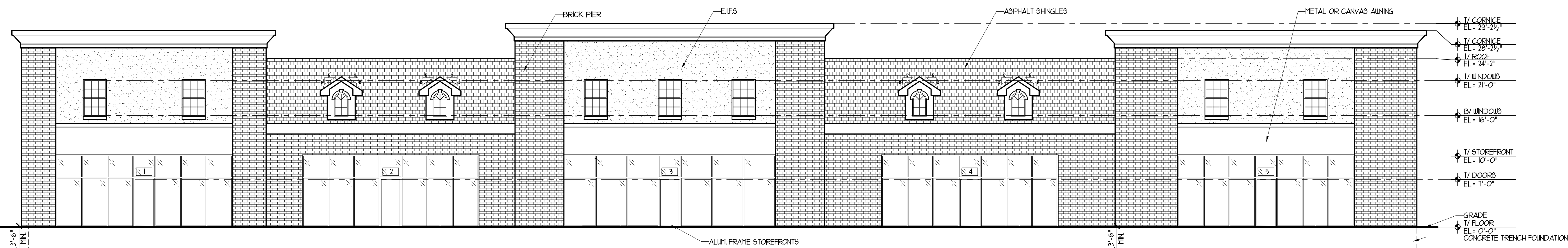
BUILDING 2 PROPOSED FRONT ELEVATION SCALE : 1/8" = 1'-0"
